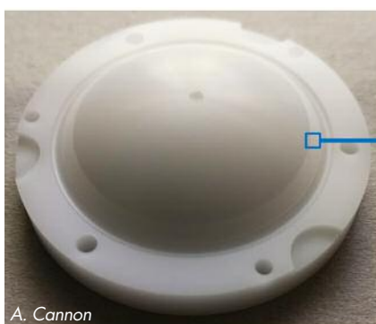
Mold (left) used to produce micro texture (right) into the edge of the suction cups.
